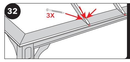
Anchor each rafter to the plate on the marked "X"s using three 3 1/2" screws, staying flush with the vertical line keeping 1/4-1/2" away from the edge of the plate.
