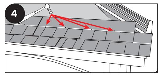
Attach second row of shingles to the roof using 5/8" roof nails provided or a power stapler. Do not use long nails or staples that protrude through 1X6 roof decking.
