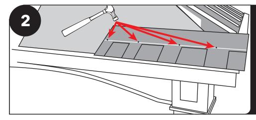
Use four 5/8" roofing nails and attach to roof through shingle at the center line marked on the shingle. Do not fasten below the line or your fasteners will be exposed.
