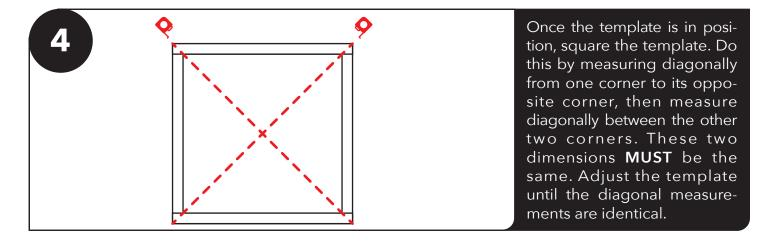
Once the template is "square", mark the post locations using the **INSIDE** corners of the framed box on the concrete slab with a pencil. After all the post locations are marked on the concrete slab, remove the wooden template. Disassemble it and set the 2x4s aside for use in step 13.
