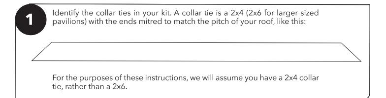
If you have only one collar tie, you will fasten it to the center rafter (skip to Step 4 on the next page). If you have more than one collar tie, space the collar ties on the ground evenly along the length of the structure, each collar tie directly below a rafter.
