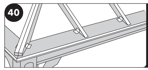
Fasten two 'A23 Simpson' brackets with 1 1/2" screws on either side of each corner hip rafter and one 'A23 Simpson' bracket at each side rafter and jack rafter. **NOTE: If you purchased an electrical package turn to page 24 for installation instructions.**
