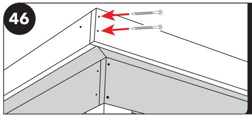
Moving to the short side, hold fascia in place, butting the top of the fascia board against a square following the pitch of the decking. Fascia should not be lower than the pitch of the roof decking; the end of the fascia should extend out to be flush with the long side fascia board.
