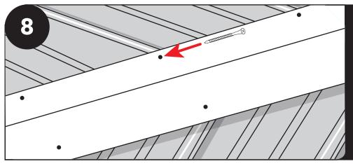
Fasten hip capping with 1 1/2" screws on the tall ridges.
