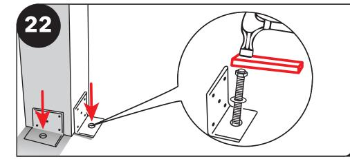
Before inserting the bolt, make sure dust is removed from hole. Then screw the nut and washer are on about 1/8" below the top of the bolt. Next, insert the wedge anchor bolt into the hole. To protect the threads and nut, tap the bolt into the ground with a piece of wood as a buffer.
