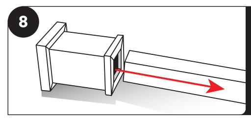
Slide your bottom post base on the post. Be sure to slide the bases up the post to make room for completing steps 9-22. NOTE: For HD High Wind brackets see bracket appendices on page 24 before moving on to step 9.
