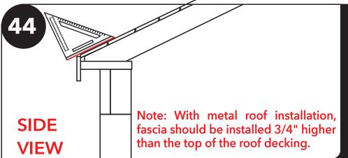
Starting on the long side, hold fascia in place butting the top of the fascia board against a square, following the pitch of the decking. Fascia should not be lower than the pitch of the decking; the end of the fascia should remain flush with the end of the plate.
