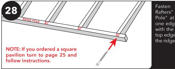
Fasten the marked "Side Rafters" to a marked "Ridge Pole" at each "X", keeping one edge of the rafters flush with the vertical line and the top edge flush with the top of the ridge pole.
