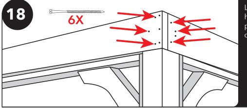
Locate 24 8" GRK screws in the hardware box. Those go in the predrilled holes at the corners of the beams. (6 per corner)
