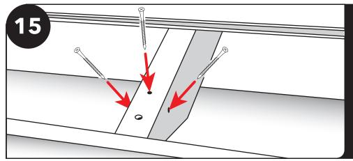
Use 2 1/2" screws to attach the rafters to the top plate. You will want to screw one screw into the top of each rafter and then another screw into the side of each rafter.
