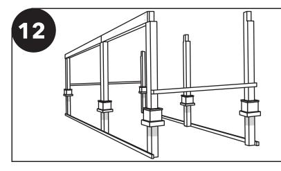
Remove template boards from the posts on the short side. Attach a template board spanning from the two corner posts on the short sides.
