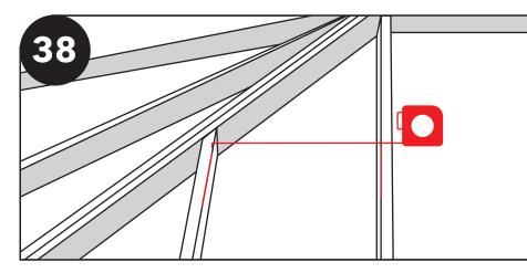
Measure from the top of the jack rafter to the side of the side rafter. Repeat the measurement on the lower end of the jack rafters before fastening to ensure equal distance at top and bottom.
