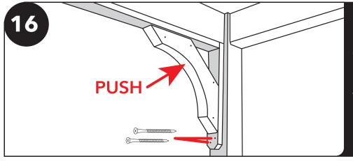
Push rail up against the bottom of the header. Put in center of post. Fasten to post with four 2 1/2" screws on both sides. Make sure the screws on the braces are turned in toward the inside of the building.
