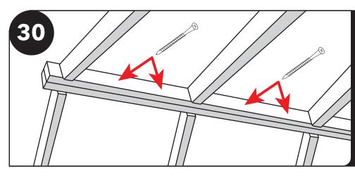
Screw the two sections together at the top with two 2 1/2" screws between every rafter. Keep ends even.
