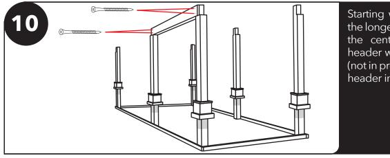
Starting with a corner post of the longest side and moving to the center post, attach first header with two 3 1/2" screws (not in predrilled holes) to hold header in place.
