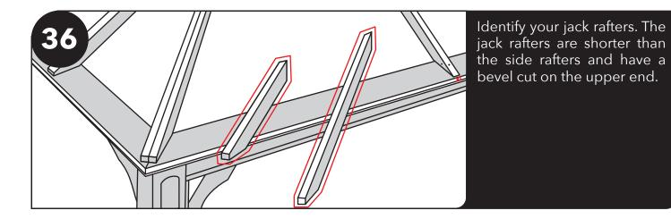
Jack rafters will only fit properly on left or right side based on upper bevel angle. Fasten correct jack rafter into the hip rafter with two 2 1/2" screws staying 1/4-1/2" in on the edge of the plate.
