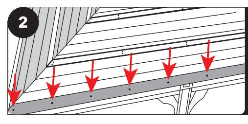
Install the drip edge over the bottom lath piece. Cut each piece to length. Fasten with 1" screws, staples, or nails every 16".
