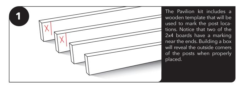
Arrange the template pieces so that they are positioned in the exact location of where the Pavilion will be placed. The boards with the marking on the end will be across from each other. The marks will show where the other boards will be attached to create this box.
