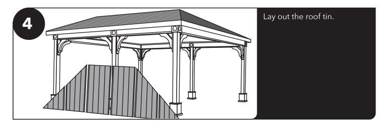
Install the tin, starting at the center and moving to each end. Ensure the first piece is installed squarely. Keep the bottom of the tin flush with the drip edge. Fasten with 1" screws. The first piece will have 3 screws at every lath.
