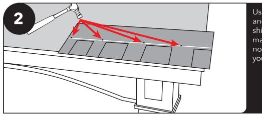
Use four 5/8" roofing nails and attach to roof through shingle at the center line marked on the shingle. Do not fasten below the line or your fasteners will be exposed.
