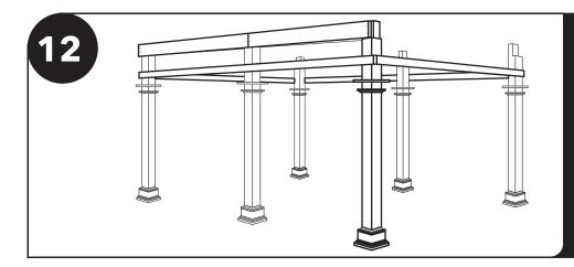
Attach short end headers with three 3 1/2" screws (in the predrilled holes) into the end of the other two beams. Repeat on opposite side with the last remaining beam.
