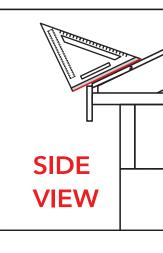
Note: With metal roof installation, fascia should be installed 3/4" higher than the top of the roof decking.
