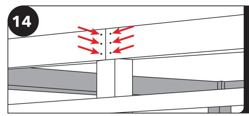
Locate the 12 GRK 4" screws. Screw three GRK 4" into left and right side of the header seam on the center post (using the pre-drilled holes). Repeat on the opposite side of the pavilion anchoring your last two beams.
