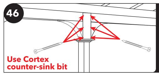
Install the inside center trim by fastening it to the top of the center post with six 2 3/4" Cortex screws into the pre-drilled holes on the face of the inside center trim.
