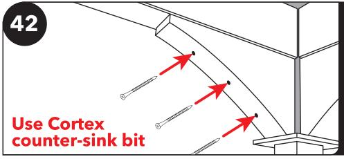
Install the bottom brace covers using three 2 3/4" Cortex screws. Continue with all 8 braces.
