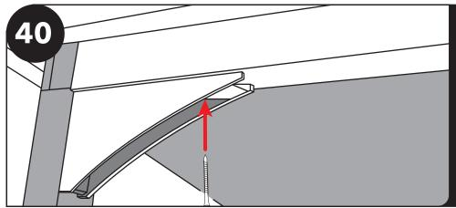
Keep the brace flush on the outside of the post. Fasten to post with two 3 1/2" screws and up into the header with two 3 1/2" screws. Line the top of the brace up with the header seam above staying 5/8" from flush. Being sure to keep the back of the brace flush with the post below.
