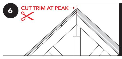
Once you have all the tin installed, hold the gable end trim in place to mark the upper end of the trim that will need to be cut to meet flush with the other side.
