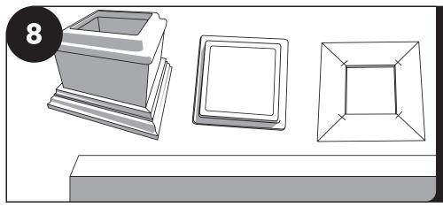
Collect post components to be placed on posts (Bottom post trim, top sleeve trim, top square trim, and post sleeve). NOTE: If you ordered an electrical package, there will be a 6X6 post with a notch in one side. Put the sleeve with the receptable on that post as you complete step
