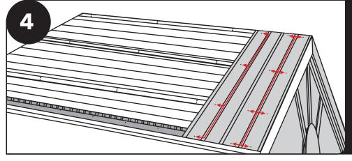
Install the tin, starting at right side and moving left. Ensure the first piece is installed squarely. Keep the bottom of the tin flush with the drip edge. Fasten with 1" screws. The first piece will have three screws at every lath.
