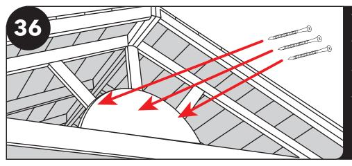
There will be two different size half-moon trim pieces. The smaller one goes on top of the fascia. The larger one fits on the inside. Fasten the half-moon trim pieces to all three boards with one 1 1/2" screw. Repeat the same process on the inside.
