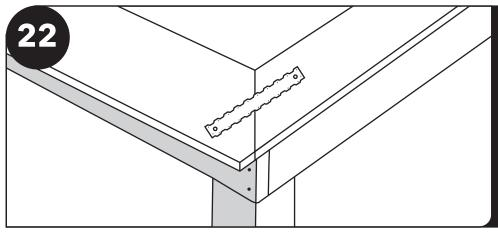
Fasten tie straps, ST2215, with 1 1/2" screws at every seam on the top of the plate.
