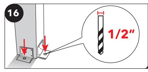
When all posts have two L brackets on, use a drill with 1/2" masonry bit to drill down about 1/2" farther than length of wedge anchor.
