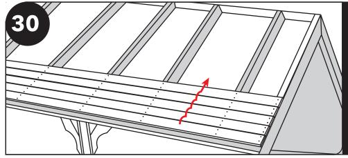
Securely interlock each piece of the roof decking, starting from the bottom and working up. Repeat step 33 on the remaining side of roof.
