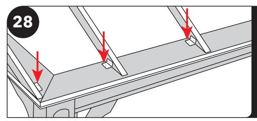
Fasten one "A23 Simpson" bracket to the side of each rafter with 1 1/2" screws. Then anchor the bracket to the plate with more 1 1/2" screws. NOTE: A23 Simpson Brackets not needed for pavilions under 16' wide.
