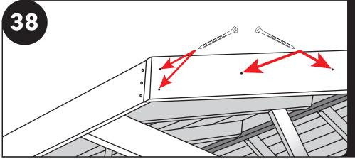
Fasten to the 2x4 rafter. One 2 1/2" screw at top and two at the bottom going into fascia. Then one every 16".
