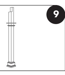
When you have all posts at marks, fasten the template boards to the tops of posts. Make sure all posts components are on, as you cannot put these on later. Make sure all posts are level and everything is square.
