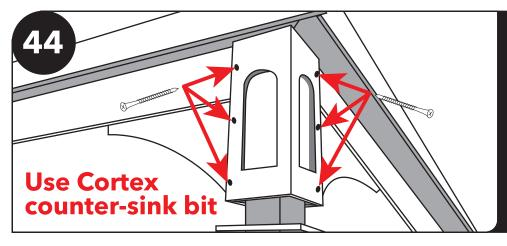
Place the outside corner trim box flush against the header and the brace, being sure that the top corner point is centered on the plate seam. Fasten with six 2 3/4" Cortex screws into the pre-drilled holes on the face of the corner trim.
