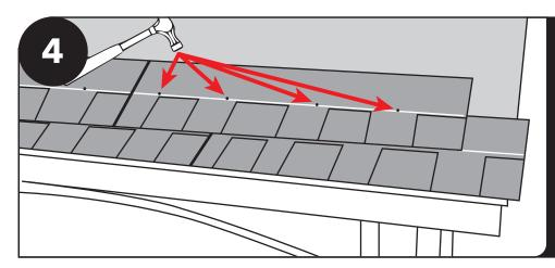
Attach second row of shingles to the roof using 5/8" roof nails provided or a power stapler. Do not use long nails or staples that protrude through 1X6 roof decking.
