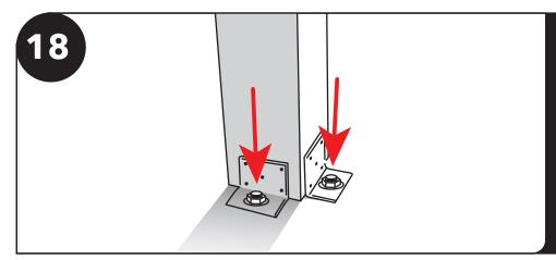
Once the wedge anchor is down against the bracket, use a wrench and tighten it down. Do that with all the anchors.
