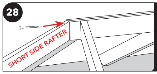
Fasten the marked "short side" rafter to the ridge pole using one 2 1/2" screw, keeping flush with top of ridge pole.
