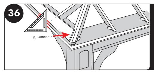
Install the first piece of roof decking making sure not to extend past plate edge. Board may need to be cut to length. (At times decking may need to be spliced on a single rafter.) Fasten decking using two 2" nails per rafter.
