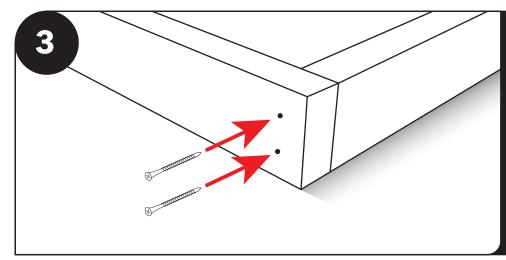
Connect the corners of the template pieces by driving two 2 1/2" screws through the side of the template boards.
