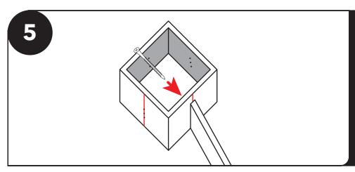
Once the rafter is properly flush. Screw the needed number of 3 1/2" screws into the pre-drilled holes.
