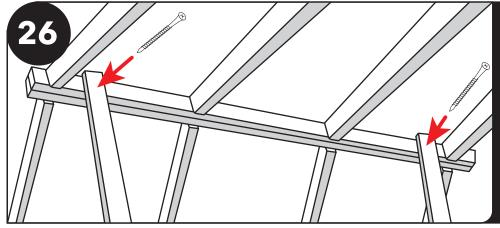
Fasten two 2x4 temporary props at either end of ridge pole to hold in place.
