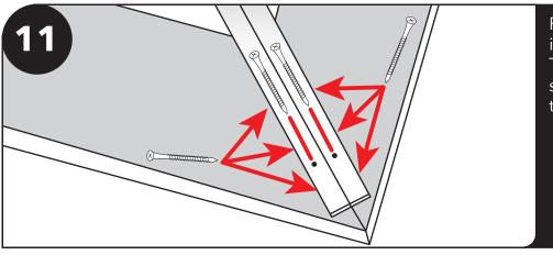
Fasten eight 3 1/2" screws into the hip rafter and plate. Three horizontally on each side and one per board on the top.
