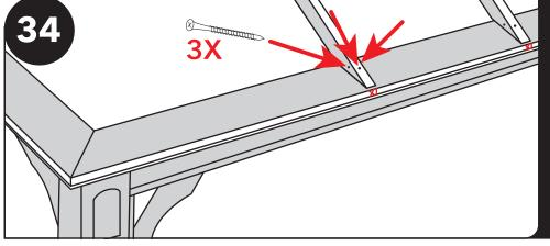
Anchor each rafter to the plate on the marked "X"s using three 3 1/2" screws, staying flush with the vertical line keeping 1/4-1/2" away from the edge of the plate.
