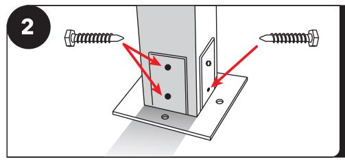
Screw the remaining six 3/8" X 3" hex lags into each post, using the pre-drilled holes. Repeat with all posts.
