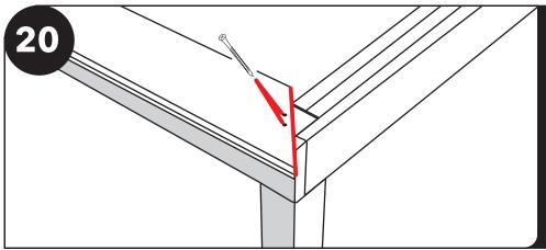
Install the four 2X12 top plates. The top plates should mount close to flush with the inside post. Make sure that the overhang is the same on both sides. Use two 3 1/2" screws to fasten the plates to the posts. Do not cut these without calling. Be sure that the vinyl side faces downward.
