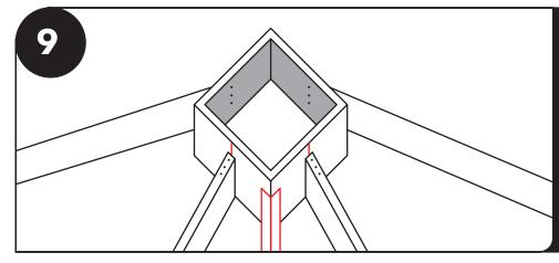
Place the 90 degree vertical notch against the corner of the compression ring. Be sure to keep the bottom edge of the hip rafter flush with the bottom edge of the compression ring. Screw 3 1/2" screws into each pre-drilled hole from the inside of the compression ring.
