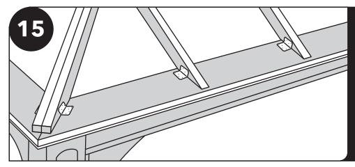
Fasten two 'A23 Simpson' brackets with 1 1/2" screws on either side of each corner hip rafter and one 'A23 Simpson' bracket at each side rafter and jack rafter.
