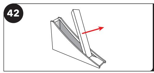
Locate the corner braces. Take the 2x4 board out from center of brace.
