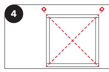
Once the template is in position, square the template. Do this by measuring diagonally from one corner to its opposite corner, then measure diagonally between the other two corners. These two dimensions **MUST** be the same. Adjust the template until the diagonal measurements are identical.
