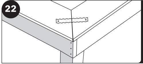
Fasten tie straps, ST2215, with 1 1/2" screws at every seam on the top of the plate.
