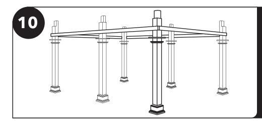
When you have all posts at marks, fasten the template boards to the tops of posts. Make sure all posts components are on, as you cannot put these on later. Make sure all posts are level and everything is square.
