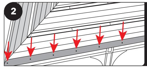
Install the drip edge over the bottom lath piece. Cut each piece to length. Fasten with 1" screws, staples, or nails every 16".
