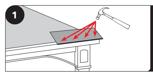
To install 1st row of shingles, turn shingle upside down with black tar line at bottom edge facing up and attach to roof using four 5/8" roofing nails. Place nails approximately 3" from bottom.
