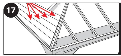
Securely interlock each piece of the roof decking, starting from the bottom and working up.
