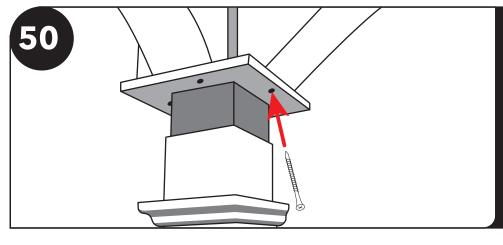
Fasten top square trim to bottom of braces with four 2 1/2" screws. Repeat on all posts.
