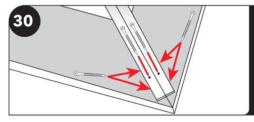
Secure the bottom of each hip rafter with six 3 1/2" screws into the corner of the plate.
