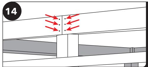
Locate the 12 GRK 4" screws. Screw three GRK 4" into left and right side of the header seam on the center post (using the pre-drilled holes). Repeat on the opposite side of the pavilion anchoring your last two beams.
