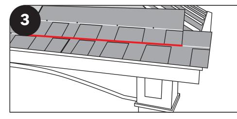
Start second row, line up bottom of shingle with the architectural line on the shingle below.
