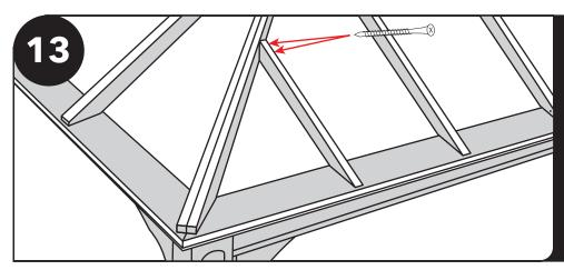
Jack rafters will only fit properly on left or right side based on upper bevel angle. Fasten correct jack rafter into the hip rafter with two 2 1/2" screws staying 1/4-1/2" in on the edge of the plate.
