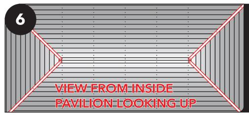
Next, install the four 1"x3" hip rafter trim pieces. Fasten with three 2 1/2" screws. Place one screw at the bottom, one in the middle, and one at the top.
