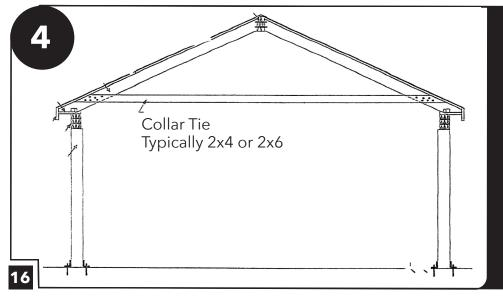
Fasten the collar tie to the rafter with six 2 1/2" screws at each end of the collar tie.
