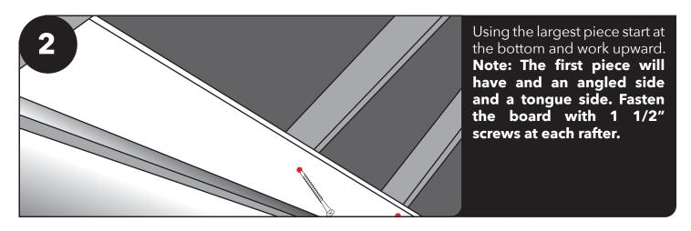
Note: Be sure that the tongue of the board is facing upward, so the next board can connect to the last.
