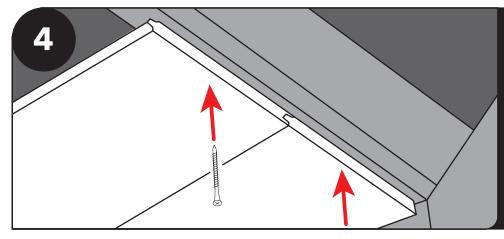
Place the groove of the next board into the tongue of the last board. Make sure boards are flush with no gaps before continuing on. Fasten board to each rafter.
