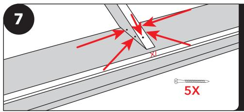
Fasten rafters centered on the marked line, located on the plate. Screw five 3 1/2" screws, two horizontally on each side and one on the top side of the rafter. Be sure to fasten each opposite side first. Do not work clockwise.
