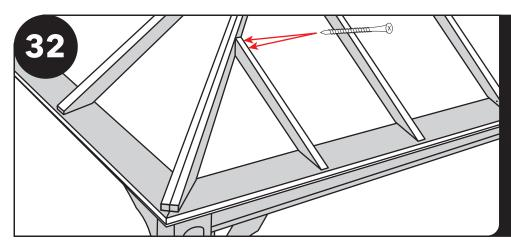
Jack rafters will only fit properly on left or right side based on upper bevel angle. Fasten correct jack rafter into the hip rafter with two 2 1/2" screws staying 1/4-1/2" in on the edge of the plate.
