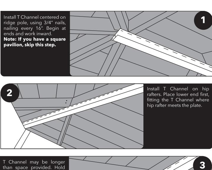
than space provided. Hold longer end against the ridge pole T Channel and mark appropriate angle then cut to size. Center on the hip rafter and fasten, using 3/4" nails, nailing every 16". Begin at the ends and work inward.
