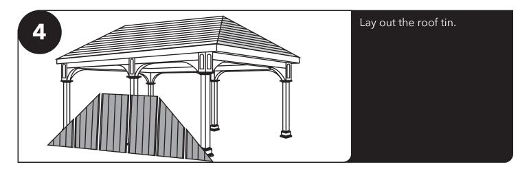
Install the tin, starting at the center and moving to each end. Ensure the first piece is installed squarely. Keep the bottom of the tin flush with the drip edge. Fasten with 1" screws. The first piece will have 3 screws at every lath.
