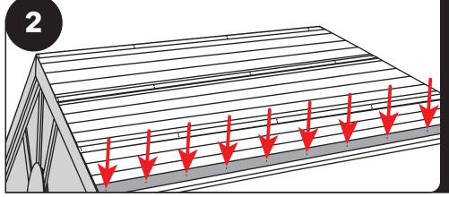
Install the drip edge over the bottom lath piece. Cut each piece to length. Fasten with 1" screws, staples, or nails every 16".
