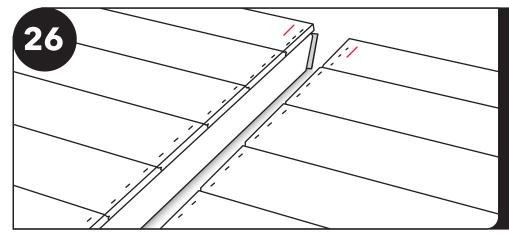
Set the roofing sections in place so the matching numbers rest against each other. The roofing sections will all be marked in the top corner with numbers.
