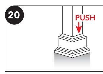
When all of the nuts have been tightened fully aand the posts are securely mounted to the concrete slab, slide the sleeve and post trim down.
