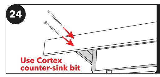
The eaves-side fascia boards will overlap the gable-sides and will extend out past them 11" (12" past the top plate). Align the pre-marked line with the end of the gable-side fascia board ends. Attach the eaves-side fascia to the top plate just as was done with the gable-sides. The eaves-side fascia will need to be connected to the gable-side fascia boards with 2 3/4" Cortex screws. Follow this process until all fascia boards are installed.
