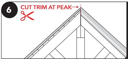
Once you have all the tin installed, hold the gable end trim in place to mark the upper end of the trim. This will need to be cut to meet flush with the other side.
