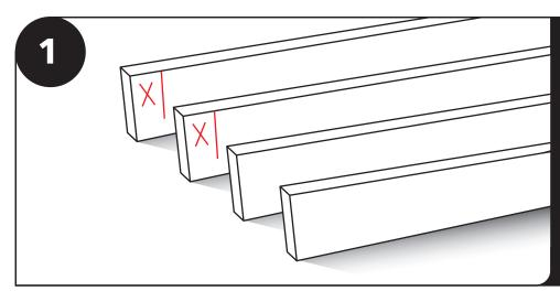
The Pavilion kit includes a wooden template that will be used to mark the post locations. Notice that two of the 2x4 boards have a marking near the ends. Building a box will reveal the outside corners of the posts when properly placed.
