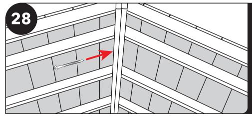
Set the first roofing section for the other side in place as was done for the first section. These two sections can now rest against each other on their ridge boards. Now, connect these two ridge boards together with one 2 1/2" screw, staggered every 16" apart. Make sure the ends of panels are flush.
