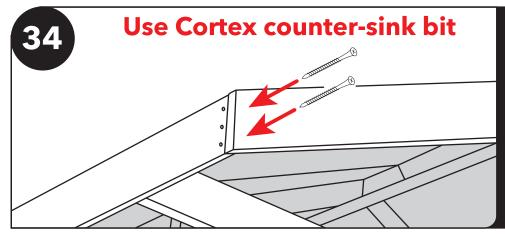
Fasten to the 2x4 rafter. One 2 3/4" Cortex screw at top and two at the bottom going into fascia. Then one every 20".
