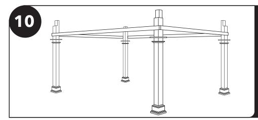
When you have all posts at marks, fasten the template boards to the tops of the posts. Make sure all posts components are on, as you cannot put these on later. Make sure all posts are level and everything is square.
