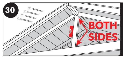
Once all the rafters are connected, install the vertical board of the gable sunburst design. Make sure it is in the center of the building. Fasten with four 2 1/2" screws. Two on top, two on bottom.
