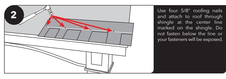
Start second row, line up bottom of shingle with the architectural line on the shingle below.
