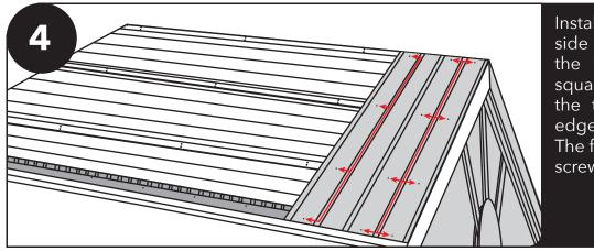
Install the tin, starting at right side and moving left. Ensure the first piece is installed squarely. Keep the bottom of the tin flush with the drip edge. Fasten with 1" screws. The first piece will have three screws at every lath.
