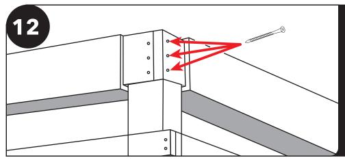
Once you have the two long side headers up, put the shorter ones on. These get fastened to other headers with three 3 1/2" screws. Use the three pre-adrilled holes going into other header.
