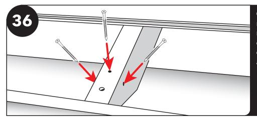
Once you have all the bottom roof decking off, screw each rafter down into plate with one 2 1/2" screw down the center and two 3 1/2" screws angled on the sides.
