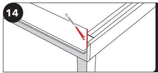
Install the top plates, vinyl side down. Position one 2x12 on the eaves side of the pavilion. Center the plate so that both ends fall at the same place on the top of the post, visually splitting the post-top from corner to corner. Be sure the overhang measurement matches on both ends. Use two 3 1/2" screws to fasten the plate. **DON'T CUT WITHOUT CALLING.**
