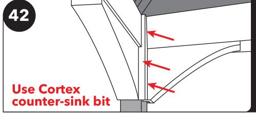
Install the inside corner trim. Fasten with three 2 3/4" Cortex screws.
