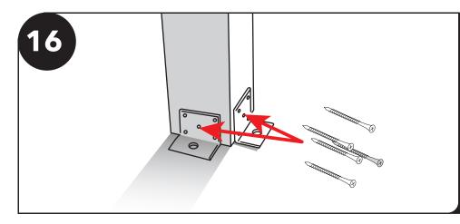
Slide the sleeve and post base trim up. Make sure the posts are all level and everything is square. Fasten two L-brackets on the outside edges of each post with five 2 1/2" screws per bracket. NOTE: For HD High Wind brackets see bracket appendices on page 21 Step 2.
