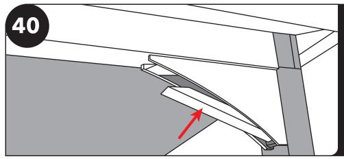
Once you have all the braces installed, put the 2x4 block back in place, fasten with two 2 1/2" screws at the top and two 2 1/2" screws at the bottom.
