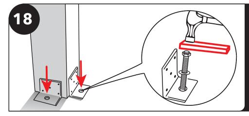
Before inserting the bolt, make sure dust is removed from hole, then screw the nut and washer on about 1/8" below the top of the bolt. Next, insert the wedge anchor bolt into the hole. To protect the threads and nut, tap the bolt into the ground with a piece of wood as a buffer.
