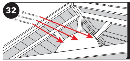
There will be two different size half-moon trim pieces. The smaller one goes on top of the fascia. The larger one fits on the inside. Fasten the half-moon trim pieces to all three boards with one 1 1/2" screws. Repeat the same process on the inside.
